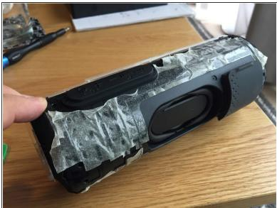
Remove the rear outer casing of the speaker.
