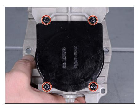
Use a Phillips #2 screwdriver to remove the four screws securing the piston cover.
