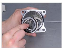
Use an angled pick to pull the washer and rubber ring 39 out of the barrel.
