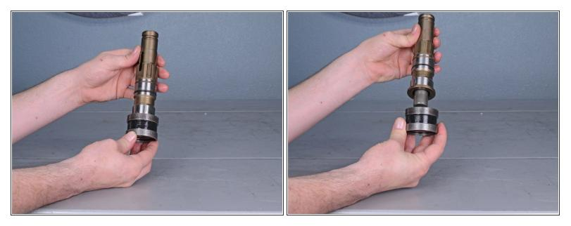
Separate the rubber ring 24 and the two metal sleeves from the bolt holder.
