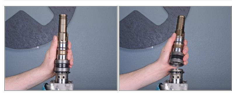
Grasp the bolt holder, rubber ring 24, and the two metal sleeves below it, and lift it off of the cylinder.
