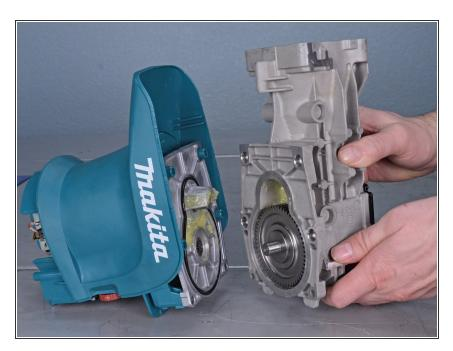
Separate the aluminum housing from the rest of the hammer.
