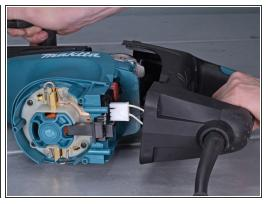
Pull the handle assembly away from the hammer, but do not completely remove it yet. It's still
