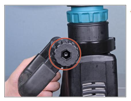
Unscrew the knob securing the side handle.
