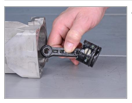
Pull the connecting rod and the piston out of the housing.
