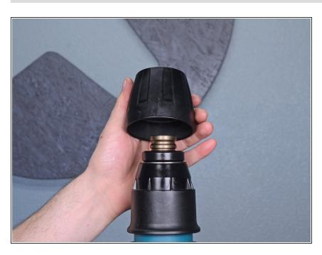
Lift the front cover off of the front of the hammer.
