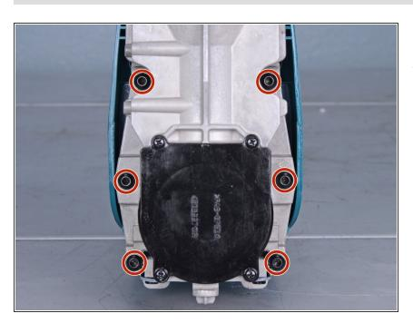
Use a 5 mm hex key to remove the six screws securing the aluminum housing.
