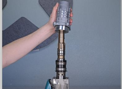
Lift the barrel straight up and remove it.
