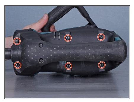
Use a Phillips #2 screwdriver to remove the six screws securing the handle assembly.
