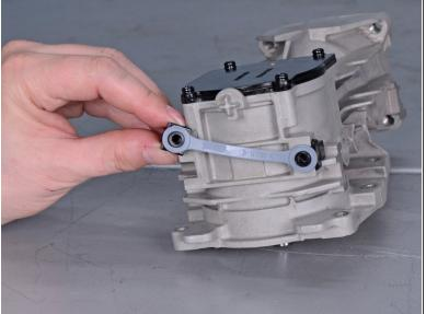
• Slide the fix guides and the rubber plate out of their slots on the housing and remove them.
