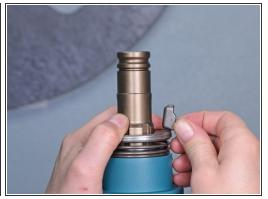
Compress the spring and hold it down while you pull the two retainers out of their slots and remove them.
