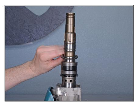
Lift the upper-most washer straight up and off of the bolt holder.
