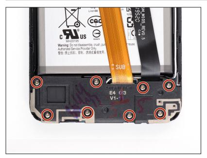
Remove the eight Phillips #00 screws from the bottom (3 mm length).
