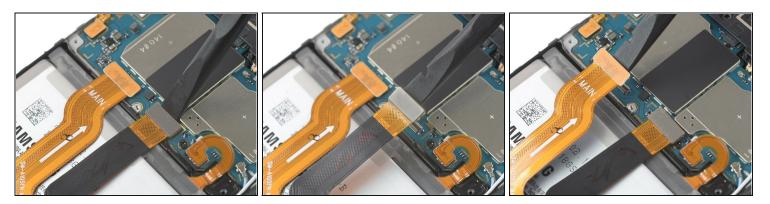
• Use the flat end of a spudger to pry up and disconnect the interconnect and display flex cables from the motherboard.
