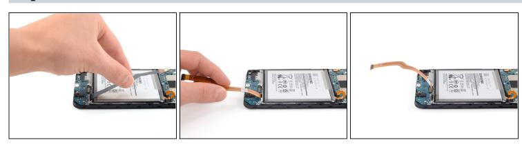
• Carefully bend the display cable away from the battery to make room for removal.
