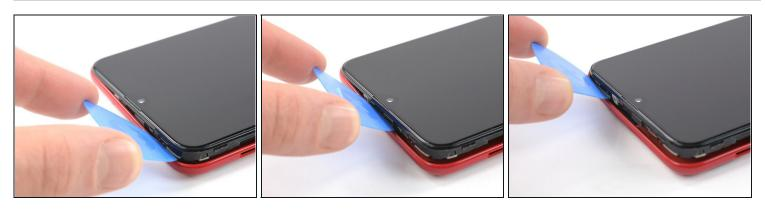
• Slide the opening pick from the top left corner to the top right corner to release the plastic clips.
