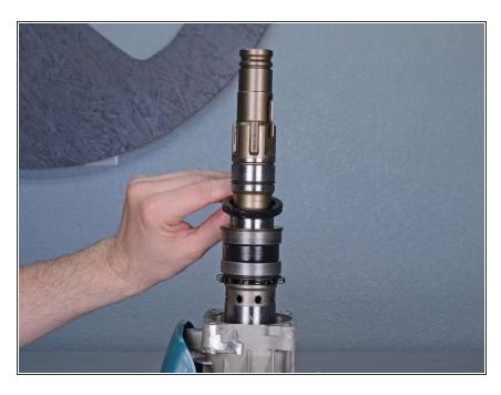
Lift the upper-most rubber ring straight up and remove it from the bolt holder.
