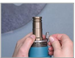
Compress the spring and hold it down while you pull the two retainers out of their slots and remove them.
