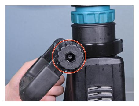
Unscrew the knob securing the side handle.
