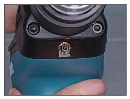
Remove the 4 mm hex bolt securing the barrel cover.
