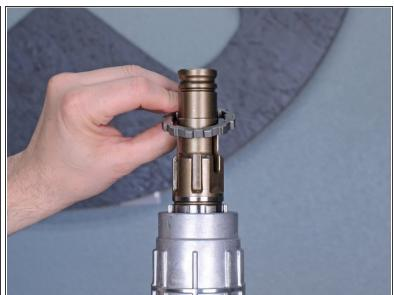
Lift the washer off of the bolt holder and remove it.
