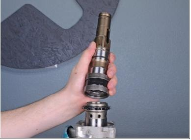
Grasp the bolt holder, rubber ring 24, and the two metal sleeves below it, and lift it off of the cylinder.
