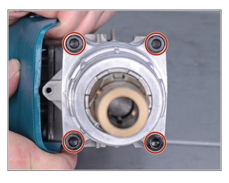
Remove four 6 mm hex bolts securing the barrel.
