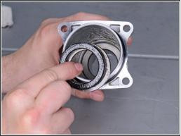
Use an angled pick to pull the washer and rubber ring 39 out of the barrel.
