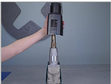
Lift the barrel cover straight up and remove it.
