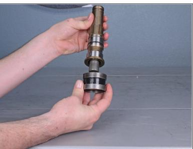
Separate the rubber ring 24 and the two metal sleeves from the bolt holder.
