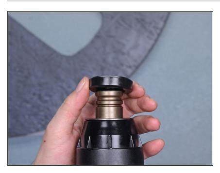
• Lift the rubber ring off of the front of the hammer.
