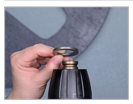
Remove the washer on the front of the hammer.
