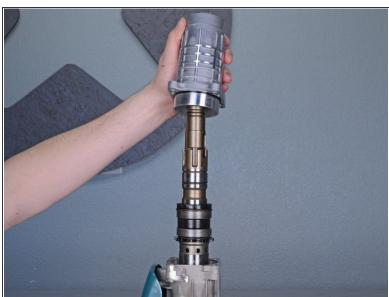
Lift the barrel straight up and remove it.
