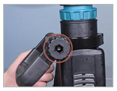
Unscrew the knob securing the side handle.
