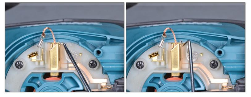
• Use a pick or small flathead screwdriver to pull the brush retaining spring off of the brush.
