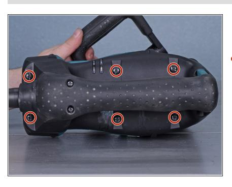
Use a Phillips #2 screwdriver to remove the six screws securing the handle assembly.
