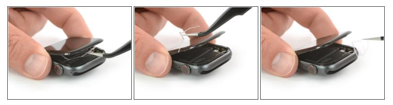
$\bigwedge$  To avoid straining the display cables, don't open the display all the way yet.
