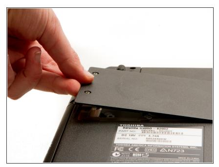
After lifting the cover up carefully, slide it to the left to be removed.
