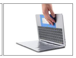
⚠ The liquid adhesive remover provided in your kit can cause damage if it contacts the MacBook Pro's display or keyboard.
