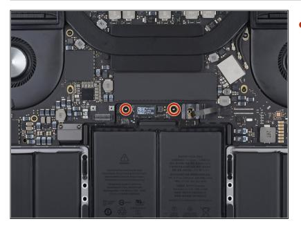
Use a T5 Torx driver to remove the two 3.2 mm screws from the battery board.
