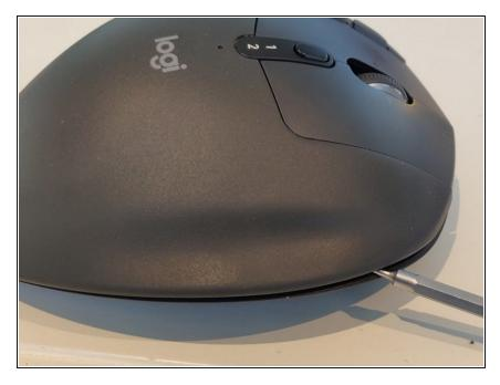
Slide a prying tool under the rightmost button and follow the seam back till the top half unclips
