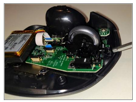
• Lever the scrollwheel sub-assembly free
