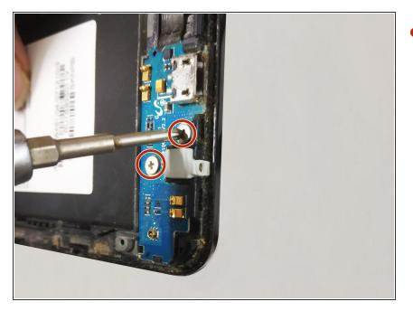
Remove the two 2.0 mm screws using the Phillips #0 screwdriver.
