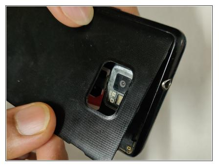
Gently remove the back cover starting from the slot given on the right side.
