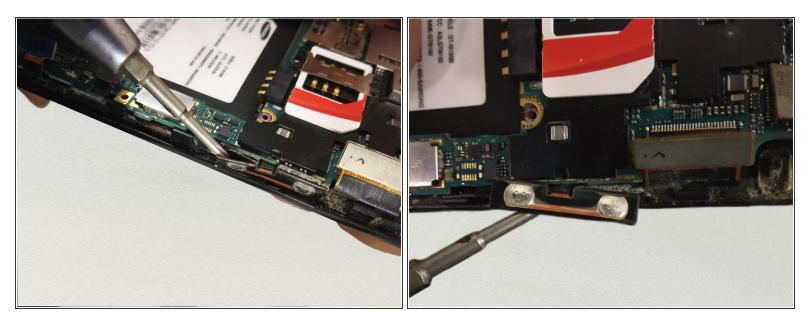
• Repeat the same procedure from step 15 to remove the volume up down button.
