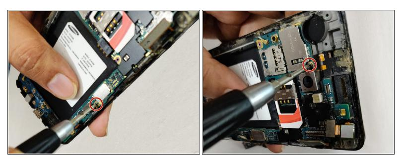
• Remove the two 1.6 mm black head screws using the Phillips #00 screwdriver.
