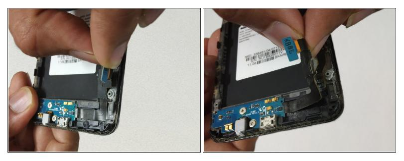
• Peel off the ribbon cable connecting the charging port and microphone by hand.
