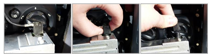
Pinch the antenna connector and pull it straight out.
