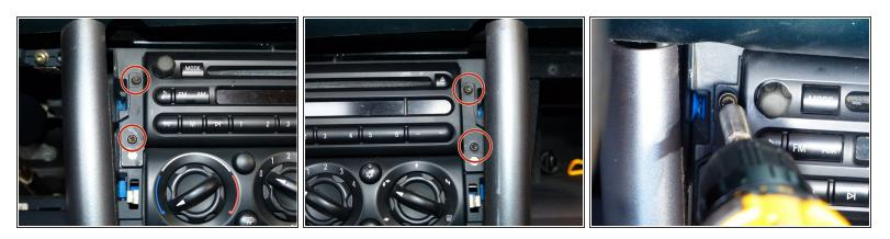
• Using a screwdriver with a T20 bit, take out the four M3 x 2 x 20 screws holding the radio in place.
