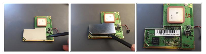
• To reveal all the components, use the spudger to lift off the metal cover of the protected circuitry
