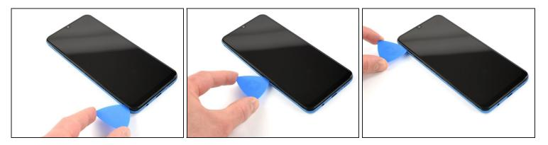
• Continue sliding the pick along the left edge of the phone to release the clips.
