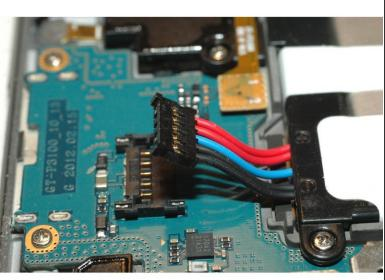
Using a non-metallic tool or your hand, detach the battery by lifting the black connector up carefully.
