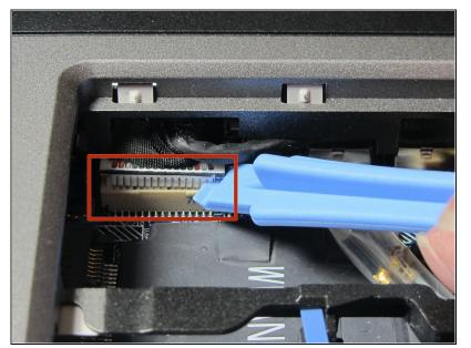
Using the spudger, unhook the touchpad's ribbon cable from the left side of the board indicated in the picture.
