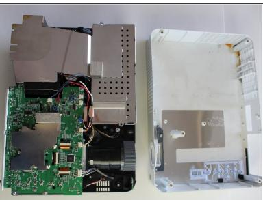
Place the projector right side up and lift the top panel up and put it to the side.
