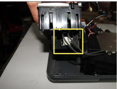
Remove two clips by pinching and pulling up on the connector.
