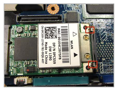
Push on the tabs indicated in the picture until the card pops up slightly then pull the card out at an angle.
