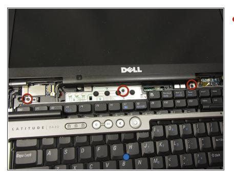
Remove the three 3mm Phillips #0 screws securing the keyboard.
