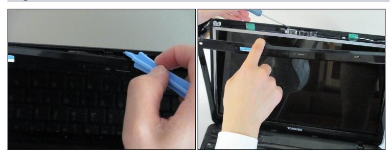
With a plastic soft pry tool, open up the laptop display assembly by methodically prying from left to right. Be careful to not damage any internal circuitry.
