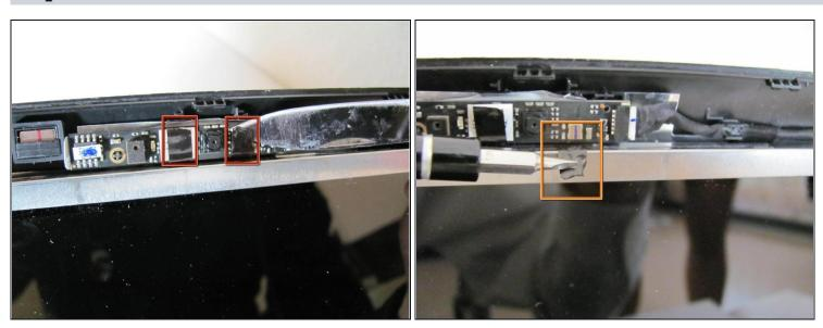
• Remove the 2 pieces of black tape using a sharp tool to free the camera board, note that the camera board is still connected to a cable.
