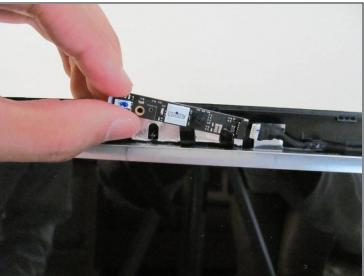
• Carefully disconnect the camera board from the laptop. We used <u>tweezers</u>.
