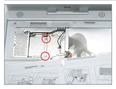
• Remove the two 2.5 mm Phillips screws that secure the RAM shield.
