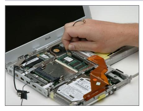
• Disconnect the inverter cable from the logic board.
