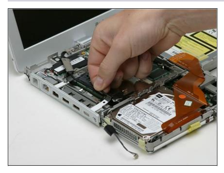
• Deroute the display data and microphone cables.
