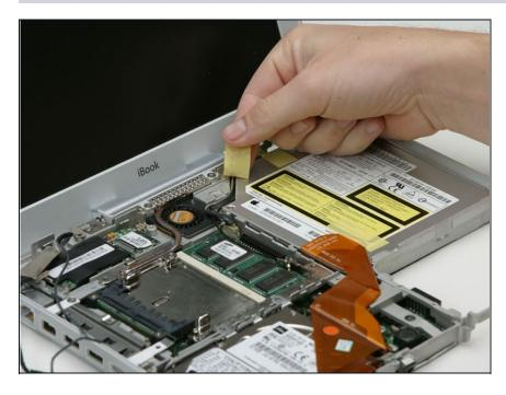
• Peel back the yellow tape securing the inverter cable to the optical drive.
