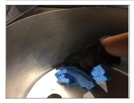
Clean the filter with soap and water and make sure to rinse thoroughly after the soap is applied with warm water. Be sure the filter is fully dried before placing it back.
