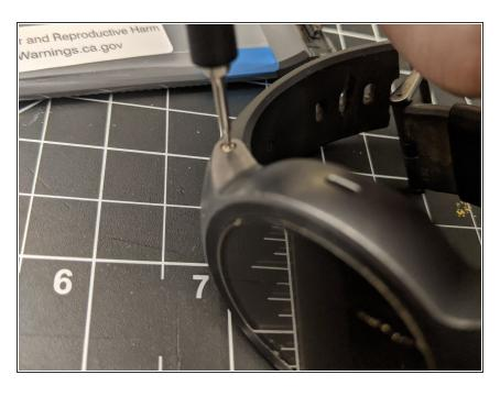
Using your Torx 4 bit, carefully unscrew the 2 screws holding in the strap. Set screws aside for later (preferably in a magnetic tray).
