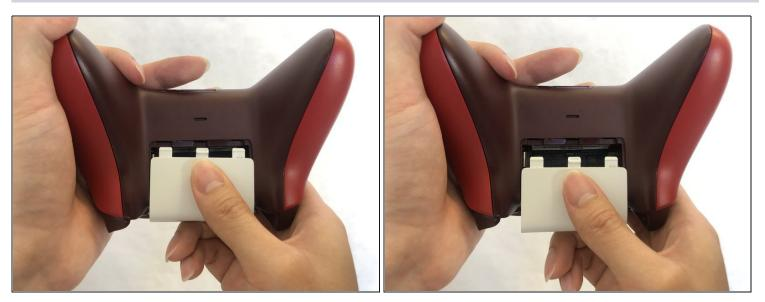
• Slide the battery cover out and remove it.
