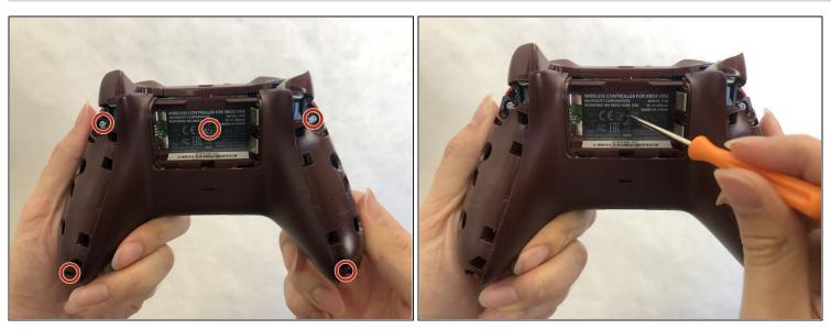
• Remove the five 2.3mm screws on the bottom plate with a T8 Torx security Screwdriver.
