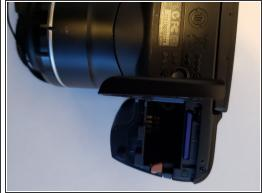
Remove the battery located at the bottom of the device.
