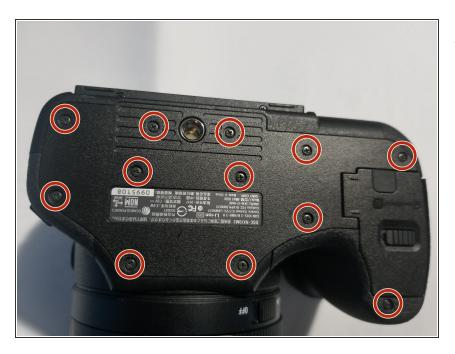
Remove the twelve 0.7mm Phillips #000 screws from the bottom case.
