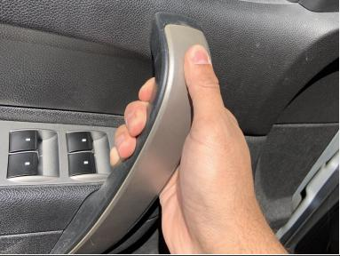
Re-attach the plastic cover by snapping it into place, start at the bottom for easier installation.
