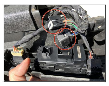
Remove all wire harnesses to the window switches from the back of the panel.
