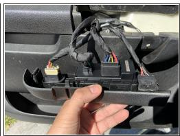
Wedge the flat-head screwdriver underneath the plastic cover to the switch panel to release it from the door.
