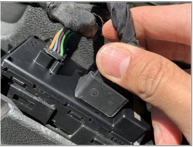
Re-plug wire harnesses into the new window switch panel and push panel into the cover.
