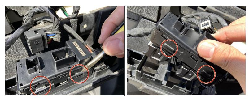
With the flat-head screwdriver release the tabs to release the window switch panel from the block of switches.
