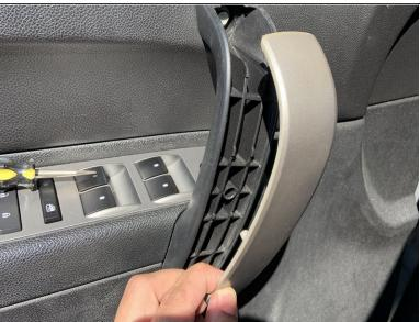
Using a flat-head screwdriver, wedge underneath the plastic cover to release it from the assembly.
