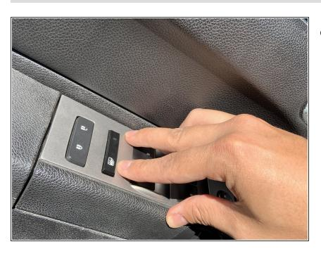
Push the re-assembled switch panel down until you hear a click, this means it is secure in the door.
