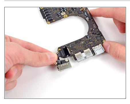
Pull the MagSafe cable connector straight out of its socket on the logic board. To reassemble your device, follow these instructions in reverse order.
