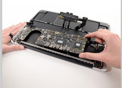
Carefully grasp the corner of the logic board (opposite of the I/O ports) and lift the logic board out of the upper case.
