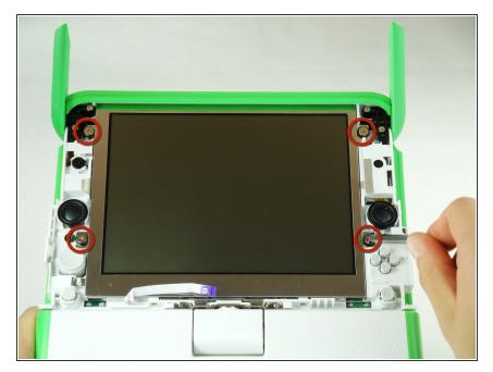
Remove the four 7.62mm screws using a Phillips #1 screwdriver.
