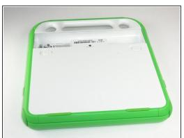
Lift the middle of the battery to remove it.
