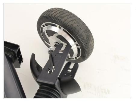
• Slide the wheel out in a downwards motion to remove it from the fork.
