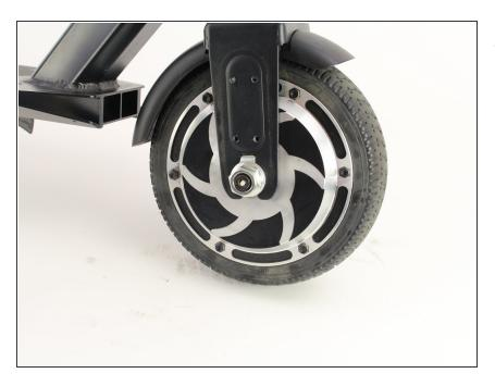
• Remove the plastic axle cover by sliding the cover downwards.
