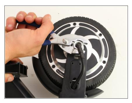
• Use pliers to remove the locknut.
