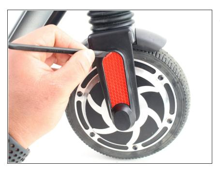
Wedge the spudger underneath the red reflective sticker and peel it back.
