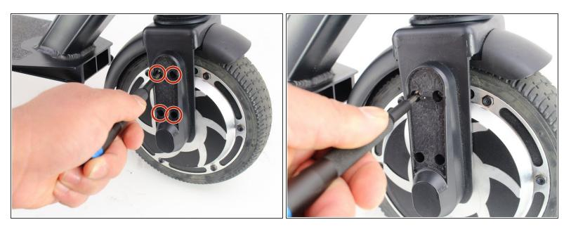
Remove the four 2mm screws with a Phillips #2 screwdriver.
