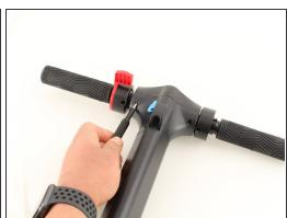
Remove the four screws from the bottom side of the display housing using a Phillips #2 screwdriver.
