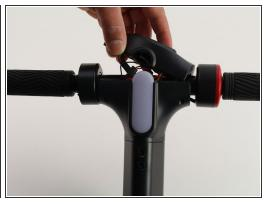
• Carefully remove the top of the housing containing the display screen.
