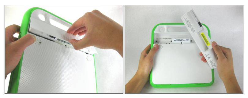
• Lift up on the middle of the battery to remove it from the device.
