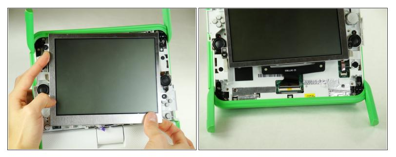
Be careful not to pull the screen out too far. There are two ribbon cables attached to the screen, and they can easily break.
