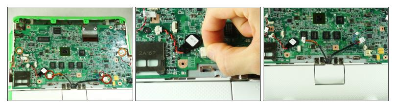
$\bigwedge$  Pull the connectors out by holding the plastic tabs and not the wires.
