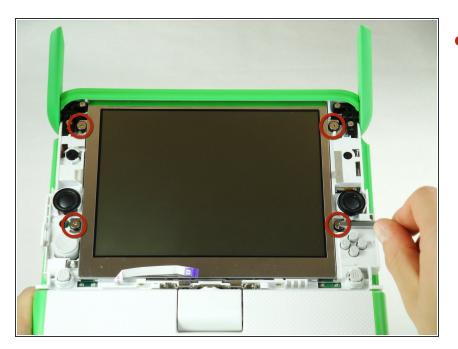
Remove the four 7.62mm screws using a Phillips #1 screwdriver.
