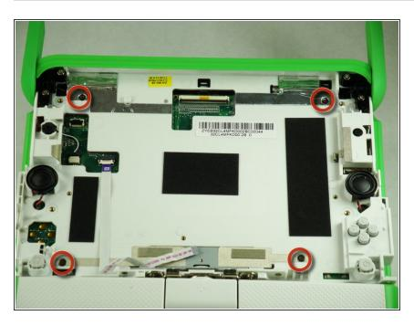
Remove the four 6mm screws using a Phillips #1 screwdriver.
