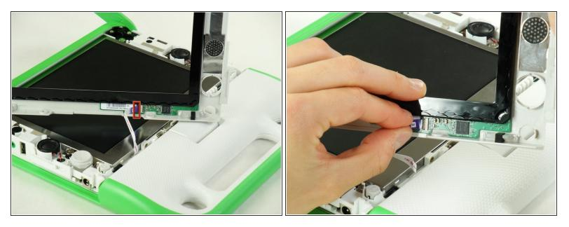
• Lift the black connector and pull the ribbon cable out by the purple tab, freeing the frame.
