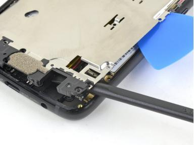
Insert the flat end of a spudger under the lower right edge of the midframe and pry up to release the midframe clip.
