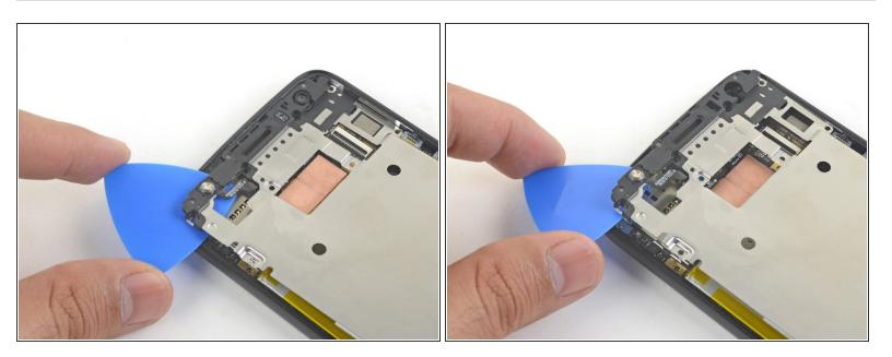
Insert the point of an opening pick under the top left corner of the midframe and twist slightly to release the top clip.
