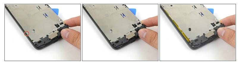
Grasp the lower edge of the midframe and pull the edge slightly to the right, to clear the metal midframe clip.
