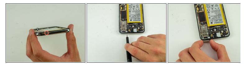
• Use the SIM card removal bit to remove the SIM card tray.
