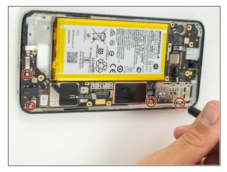
Use a T3 Torx screwdriver to remove the four 2.3mm screws from the bottom and right sides of the phone.
