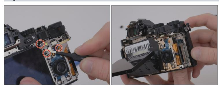
• Place the tweezers on the side of the circuit board and lift it from underneath so as to free it from the three retaining tabs.
