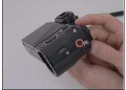
Remove the six M1.5x4mm screws with a PH00 Phillips screwdriver.
