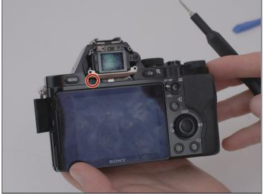
• Remove the four M 1.5x2mm screws.
