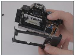
• Once the screws have been removed, unsnap and lift the rear plastic cover off of the camera.
