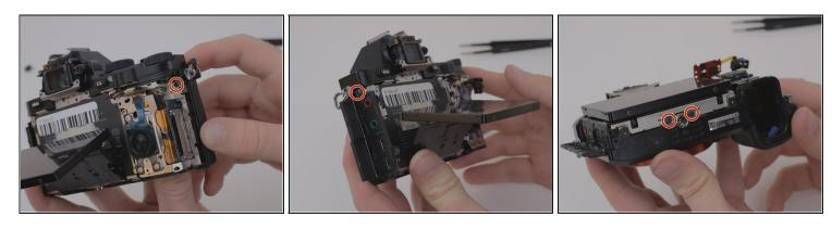
• Remove four M1.5x4mm screws using a PH00 Phillips screwdriver.
