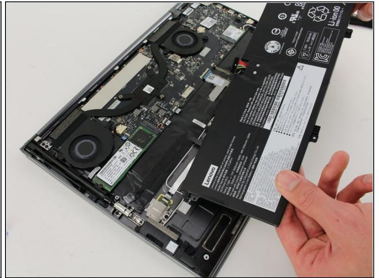
① The battery is still held in place with two stretch-release adhesive strips, [similar to ones found in an iPhone](#).
