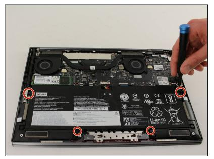
• Unscrew the four 3mm screws with a Phillips screwdriver.
