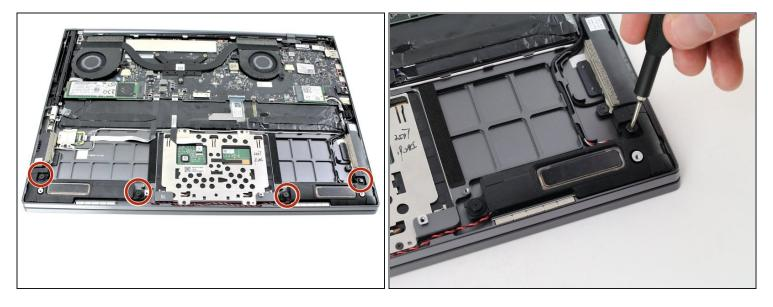
• Remove the four 2mm screws that attach the speakers to the laptop body using a Phillips #00 screwdriver.
