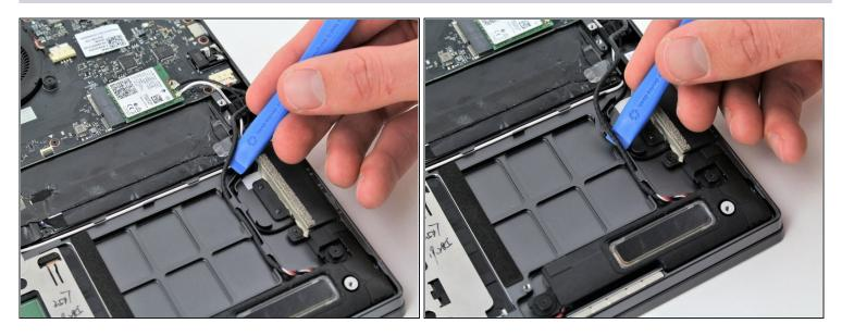
• Lift the black wire that connects the speakers to the motherboard from its track using an opening tool.
