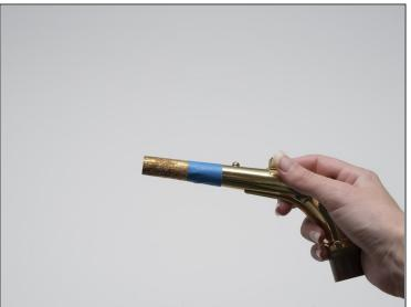
• Apply masking tape where there is no glue on the neck-piece to prevent damage to the finish.
