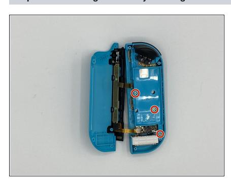
Remove the three (3) 3½mm golden Phillips #00 screws from the midframe.
