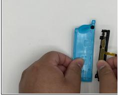
Remove the screw holding the rail in place. Remove the rail from the back frame and set it off to the side.
