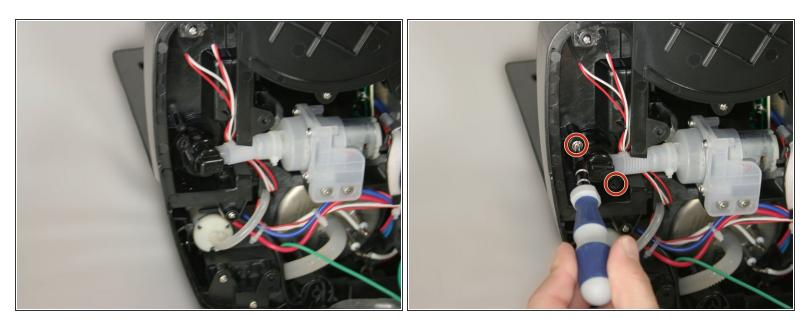
• Remove the two silver 4mm Phillips #2 screws that hold the water pump in place.
