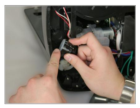
• Realign the rubber gasket of the water pump to create a tight fit.
