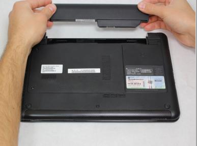
Slide the battery away from the device to remove.
