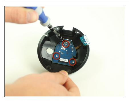
Use a T6 Torx screwdriver to undo the three 0.8 mm screws holding the inner dome daughterboard in place.
