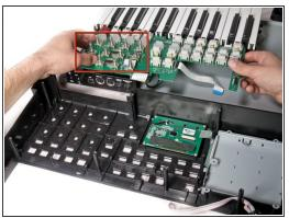
Remove the mother board completely from the face plate and identify the broken potentiometer.
