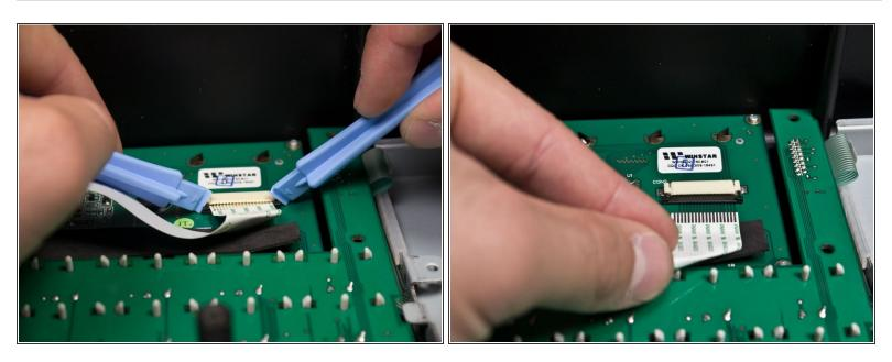
Using two plastic opening tools, slide the black locking mechanism on the ZIF connector towards you. This will remove the ribbon cable connecting the motherboard to the screen.
