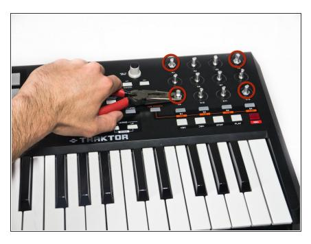
Using needle nose pliers, remove the washers from the four corner selector knobs.
