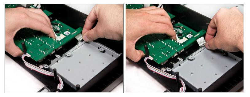
Wiggle and pull out the ribbon cable connecting the mother board to the beat pads.
