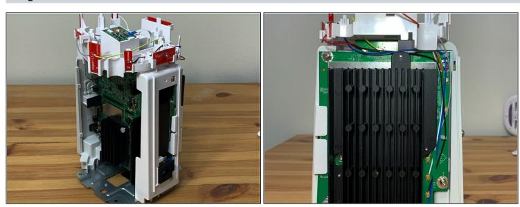
• A large heatsink on the back of the unit serves to keep the unit cool without a fan.
