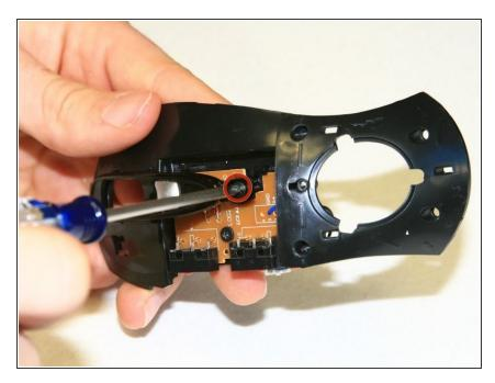
Using the Phillips #1 screwdriver, unscrew the 5 mm black flat head screw that's securing the scroll wheel cage.
