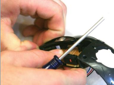
Pinch the cage to release snaps. You can now pull the cage off.
