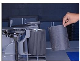
Pull the sandpaper loop straight up and remove it from the drum.
