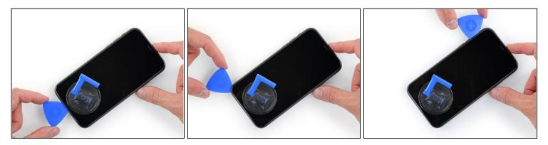
• Slide the opening pick around the lower left corner and up the left edge of the iPhone, slicing through the adhesive holding the display in place.
