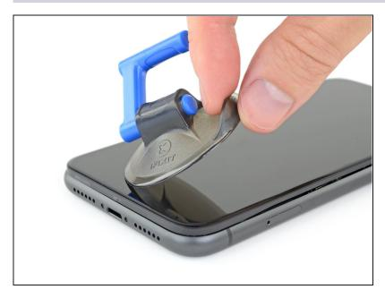
• Pull the small nub on the suction cup to detach it from the front panel.
