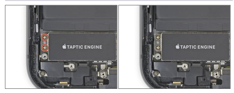
• Use a Phillips driver to remove the two 1.8 mm screws securing the Taptic Engine.
