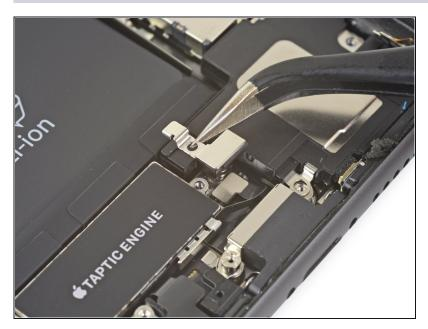
• Remove the Taptic Engine connector cover.
