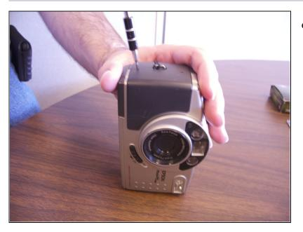
• Remove 2 screws on the rounded side of the camera wisdom here.
