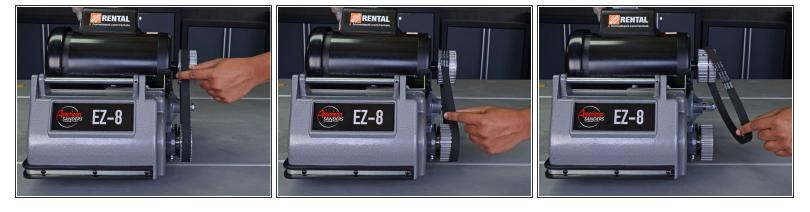
To remove the drum belt, pull it away from the sander while hand turning the belt on the drum pulley in a counter-clockwise direction. The belt will come off after a few rotations.
