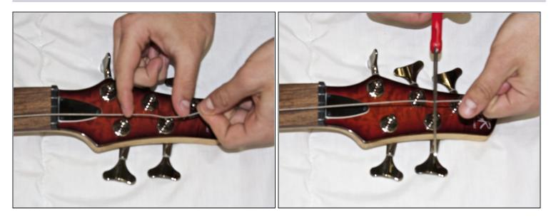
• On a taut string, measure one inch past the nut before using a pair of wire cutters to cut the string.
