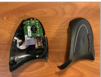
Once the three screws that are visible from the top are removed you can pry loose the side panel.
