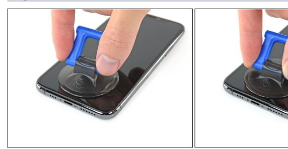
• If you're using a single suction handle, apply it to the bottom edge of the phone, while avoiding the curved portion of the glass.
